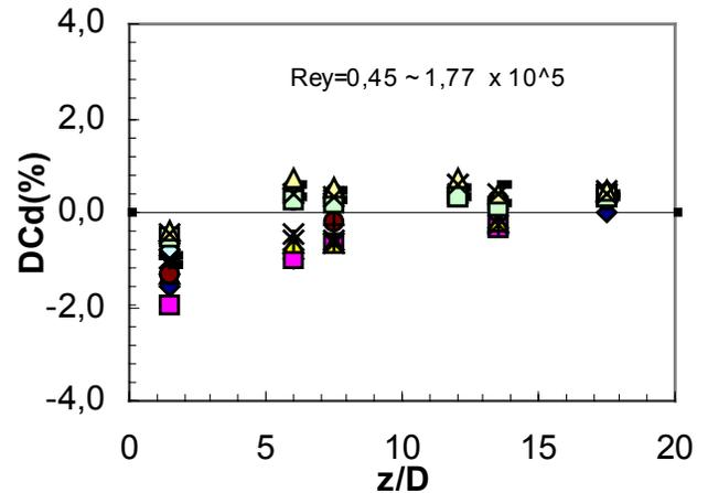
Figure 12. Discharge coefficient error downstream double bend with tube bundle flow conditioner,  $\beta=0.50$ .
