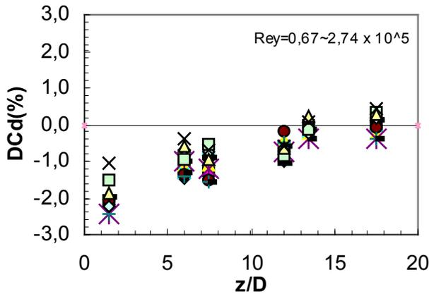
Figure 9. Discharge coefficient error downstream double bend with tube bundle flow conditioner,  $\beta=0.62$ .
