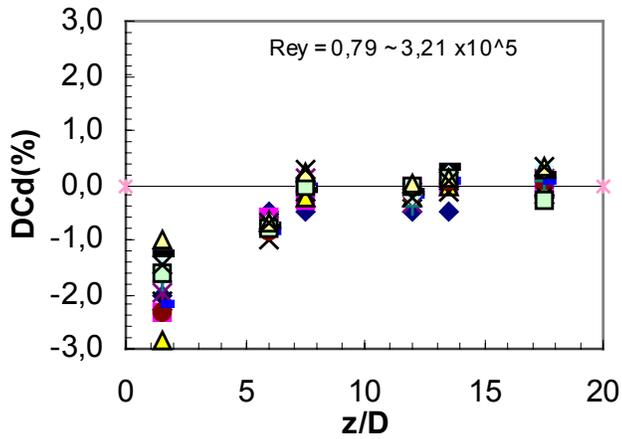
Figure 5. Discharge coefficient error downstream double bend with Etoile flow conditioner,  $\beta=0.70$ .
