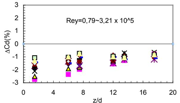
Figure 3. Discharge coefficient error downstream the double bend without flow conditioners in line,  $\beta=0,7$ .
