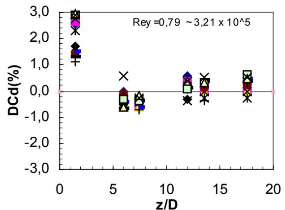
Figure 4. Discharge coefficient error downstream double bend with perforated plate flow conditioner,  $\beta=0.70$ .
