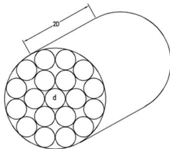
Figure 2-c. Tube bundle straightener
