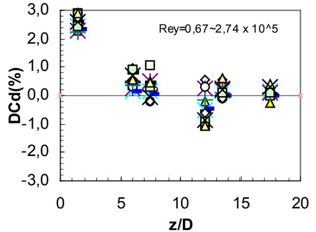
Figure 7. Discharge coefficient error downstream double bend with perforated plate flow conditioner,  $\beta=0.62$ .
