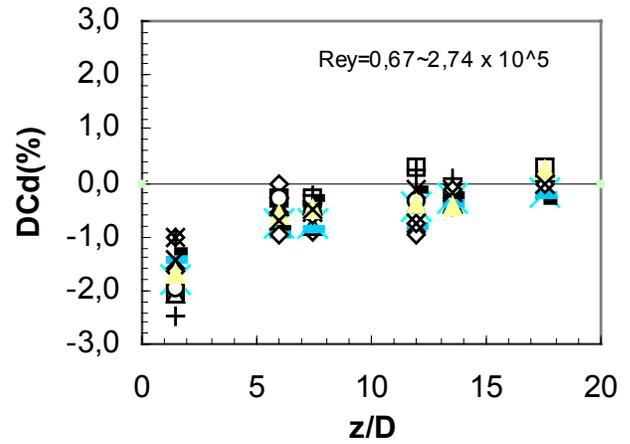
Figure 8. Discharge coefficient error downstream double bend with Etoile flow conditioner,  $\beta=0.62$ .
