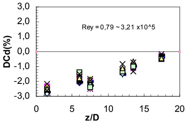
Figure 6. Discharge coefficient error downstream double bend with tube bundle flow conditioner,  $\beta=0.70$ .
