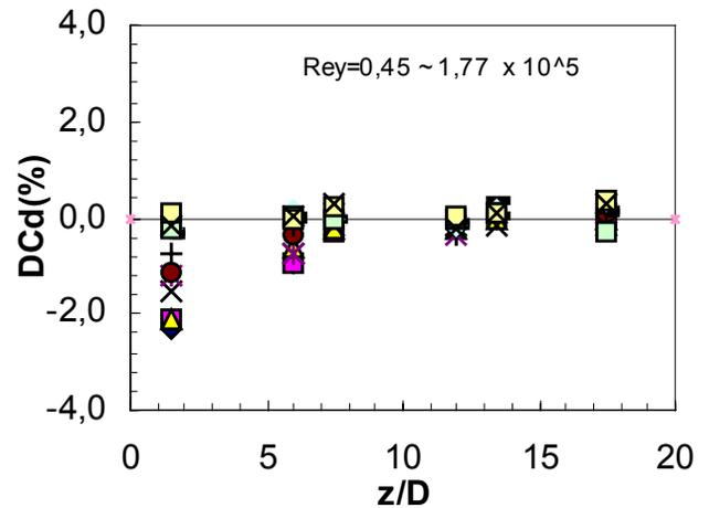
Figure 11. Discharge coefficient error downstream double bend with Etoile flow conditioner,  $\beta=0.50$ .
