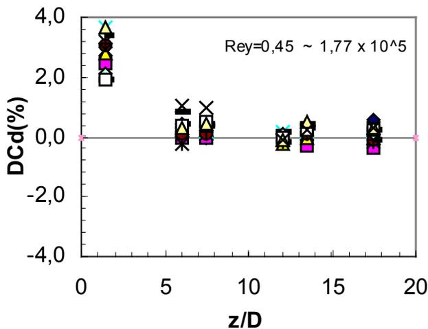
Figure 10. Discharge coefficient error downstream double bend with perforated plate flow conditioner,  $\beta=0.50$ .
